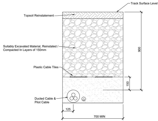
**TRENCH CROSS SECTION - PILOT CABLES**
